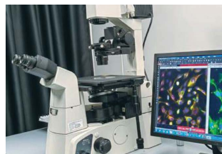
Microscopes fitted with digital camera Visualise biological sample by either taking images or capturing cellular activity on video.
