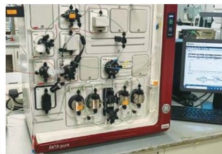
AKTA Pure Chromatography A flexible entry system that can be used for a wide variety of fast purification of peptides, proteins and nucleic acids.
