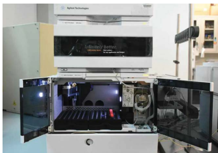
High Performance Liquid Chromatography Sophisticated instrument to separate and identify biological components in a mixture.
