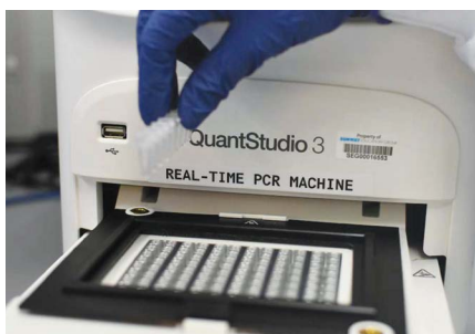
Real-Time Quantitative PCR The most sensitive technique for mRNA detection and quantification. Mostly used for molecular diagnostics and targeted gene expressions.
