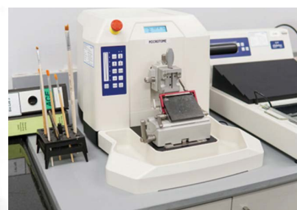
Precision Microtome Used to make thin slices of tissue for microscopy observation.
