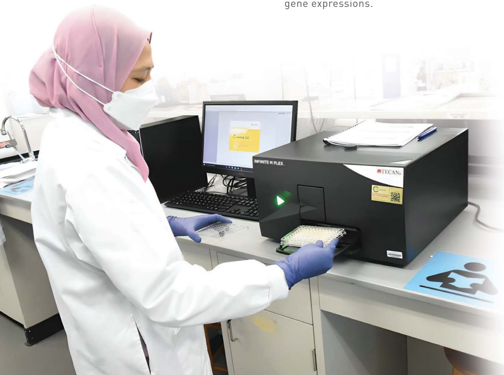
Microplate reader Analysis of biochemical and cell-based assays. Application can be ranging from basic ELISA to high throughput detection such as absorbance, fluorescence and luminescence.
