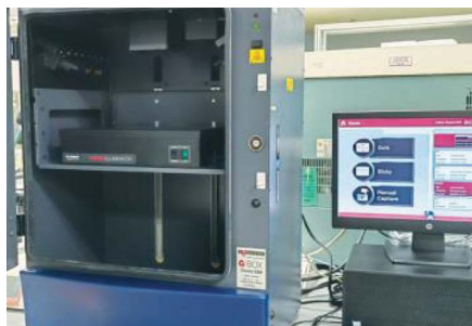
High resolution gel imaging To capture high quality agarose and protein gels for visualisation and quantification of biological samples.
