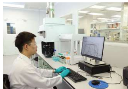
Inductively Coupled Plasma Optical Emission Spectrometer (ICP-OES)
