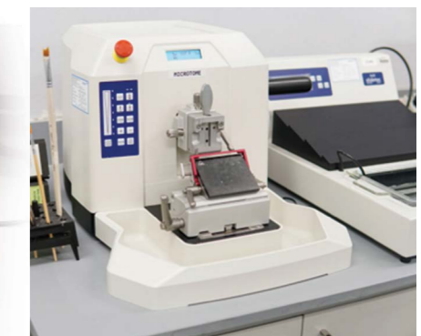
Precision Microtome Used to make thin slices of tissue for microscopy observation.
