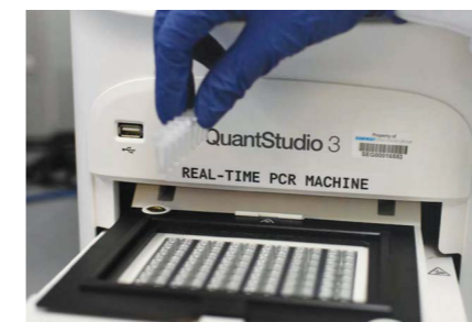
Real-Time Quantitative PCR The most sensitive technique for mRNA detection and quantification. Mostly used for molecular diagnostics and targeted gene expressions.
