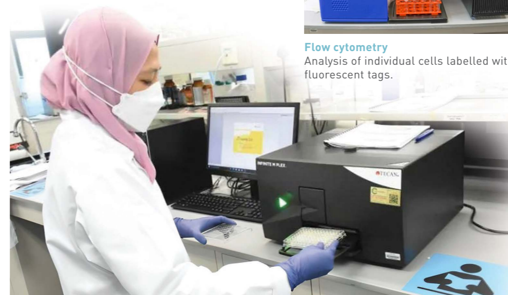
Microplate reader Analysis of biochemical and cell-based assays. Application can be ranging from basic ELISA to high throughput detection such as absorbance, fluorescence and luminescence.
