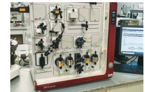
AKTA Pure Chromatography A flexible entry system that can be used for a wide variety of fast purification of peptides, proteins and nucleic acids.
