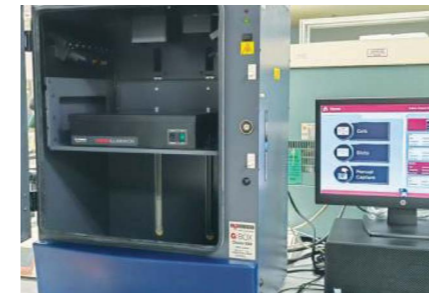
High resolution gel imaging To capture high quality agarose and protein gels for visualisation and quantification of biological samples.
